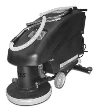
A tight turning radius and scrub head lock-down feature allow the mid-sized Wrangler 2016 to tackle heavy scrub and standard scrub jobs with ease. Its 20-in. scrubbing path makes quick work of any task. A rugged, rotocast-polyethylene body and 7-gauge steel frame deliver long term durability.
